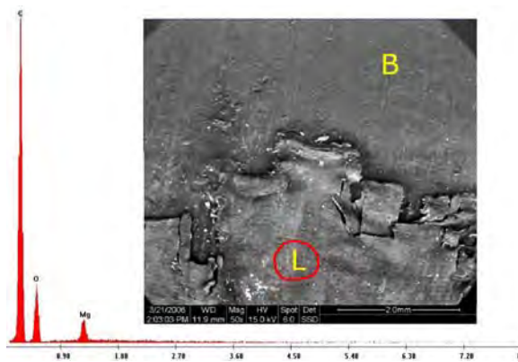
Figure B.3 SEM analysis lacquer layer zone, picture courtesy of [17].
