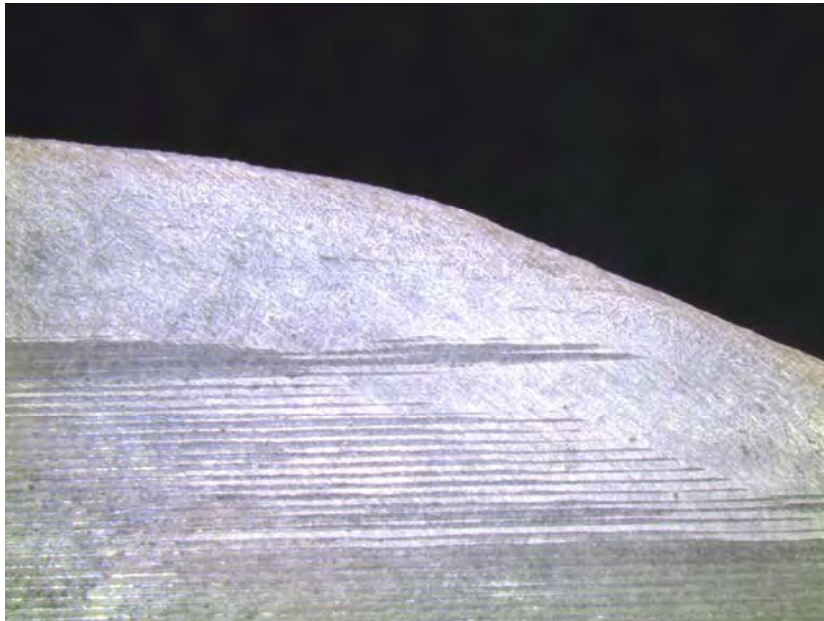
Figure 3.4 The transition from inlet to work zone photographed of a cross section of a residual billet.
