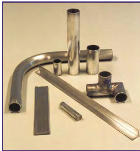
Figure 1.2 Magnesium hydrostatic extrusion products, picture courtesy of Hydrex Materials B.V.
